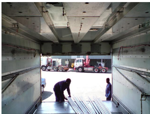
Older truck showing overhead ducting with top down recycled air pattern.
