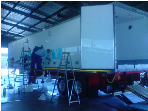
Preparing wall panels for signage.
