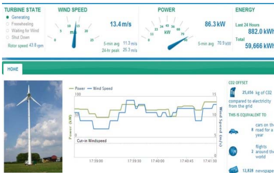
Photo 13: Monitoring performance of the Endurance turbine on-line
