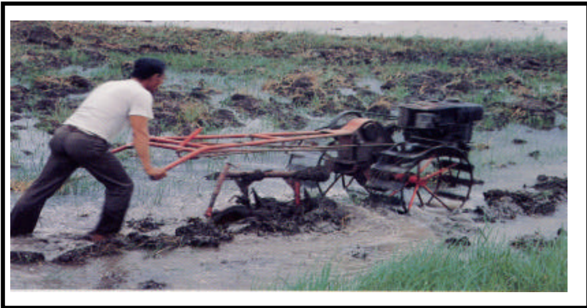
Figure 1.3 (a) Transmission system for walking tractor / power tiller (b) Walking tractor being used for ploughing flooded soil Reproduced with permission of International Rice Research Institute
