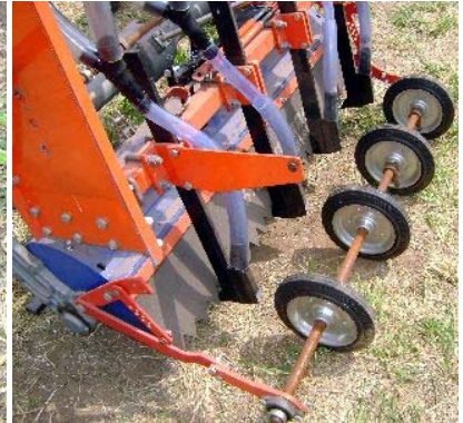
Fig 13. VMP seed and fertilizer delivery
