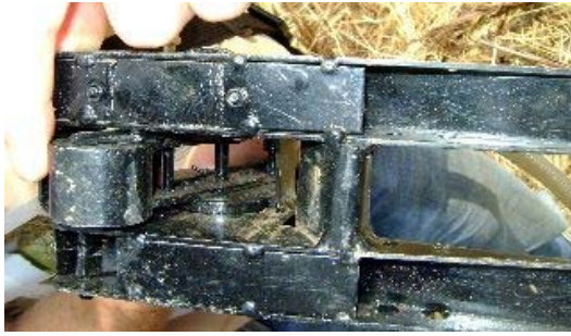
Fig. 20. Yunfan jab planter seed and fertilizer beaks and actuating pendulum
