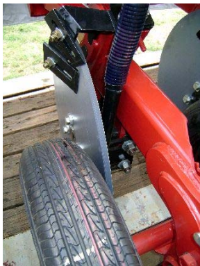
Fig. 18. 'Daybreak' single disc opener technology
