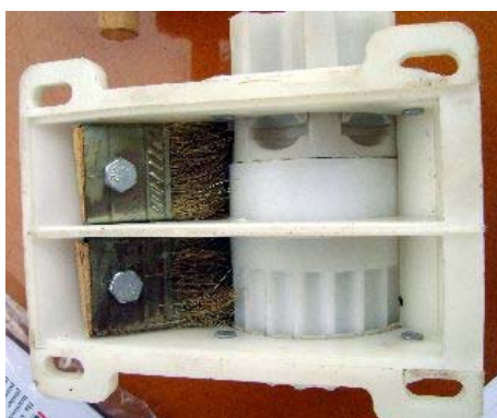
Fig. 3. Seed (cells) and fertilizer (fluted) metering
