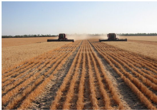
Fig. 21. the permanent wheel tracks required for CTF create better cropping conditions in the permanent beds. Machinery widths have to match the (usually 3 m) bed widths and it is best to start with the combine header as this is the biggest, heaviest and most expensive machine. Source: Don Yule
