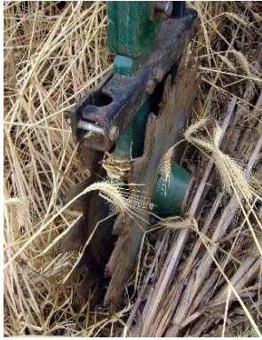
Fig. 17. Stubble Star double disc opener
