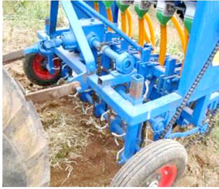
Figs 15 and 16. The chain-powered residue manager which clears residue in front of the double disc opener of the no-till seeder. Source: Li et al. , 2011. (1: tine opener; 2: Rigid fingers; 3: Chain; 4: press wheel; 5: Double disc opener)
