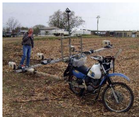
◀ Fig.26. Electrical conductivity and GPS mounted on a motor cycle ▶ Fig. 27. Helicopter with on-board camera for field mapping and problem identification
