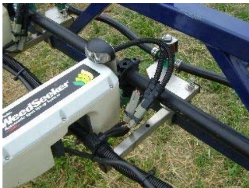
Fig. 24. 'WeedSeeker' emitter / receptor mounted forward of the spray nozzle
