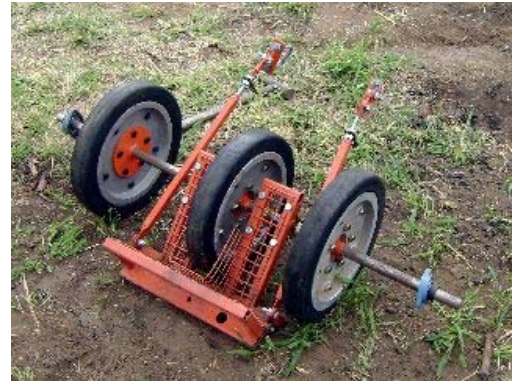
Fig. 7. Rear foot stand for better penetration
