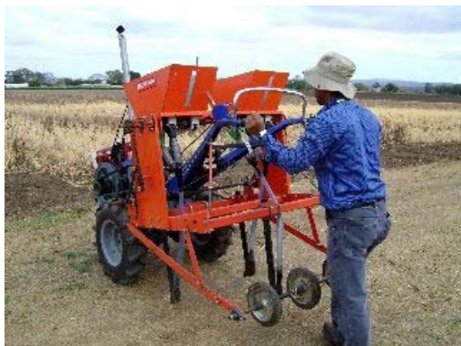
Fig. 1. ACIAR-Rogro tined seed drill
