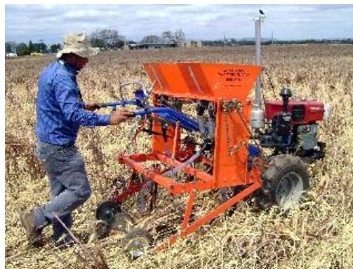
Fig. 2. ACIAR-Rogro seeding in wheat residue
