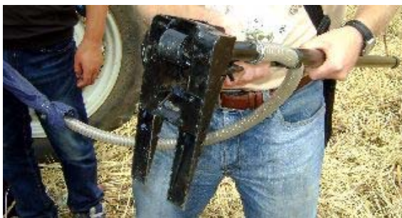
Fig 19. Yunfan jab planter. General view showing the handle / seed hopper, fertilizer bag and delivery tube
